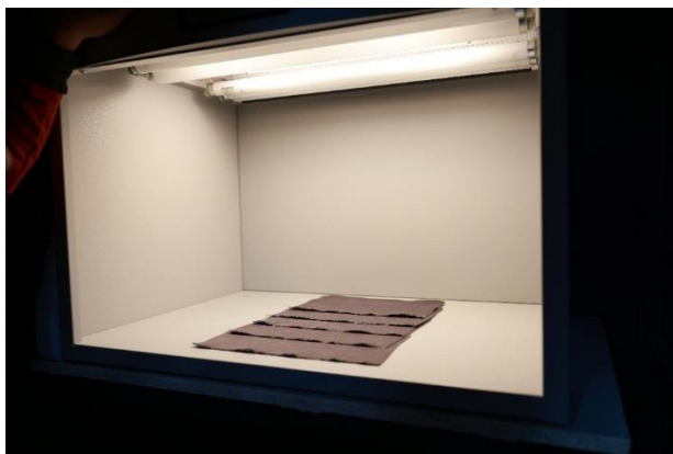
Slika 3.9. Color Light Box / Color Matching Cabinet
