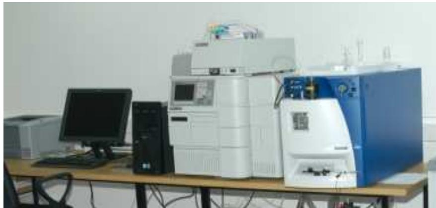
Slika 27. Sistem instrumenata HPLC/MS/MS-PDA
